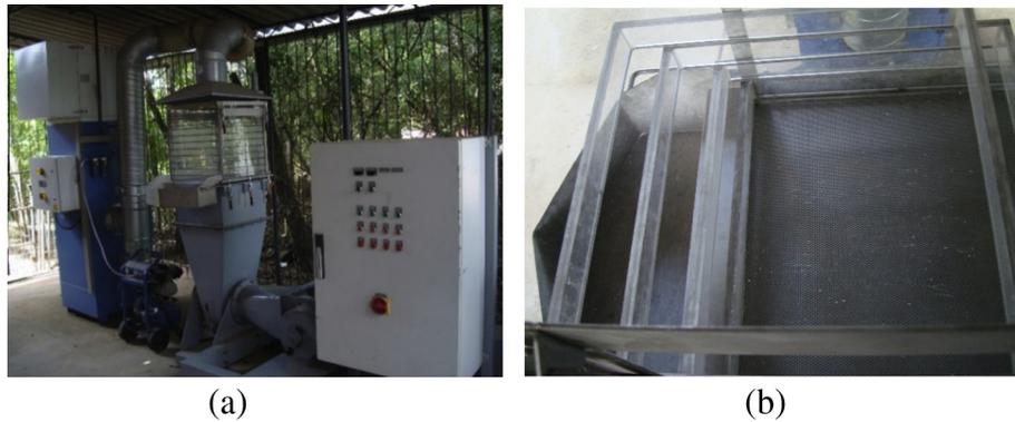
**Fig. 2.** AllMineral jig – (a) modell “AllAir S 500<sup>®</sup>”, used in the tests. (b) Assembly of the jig chambers.
